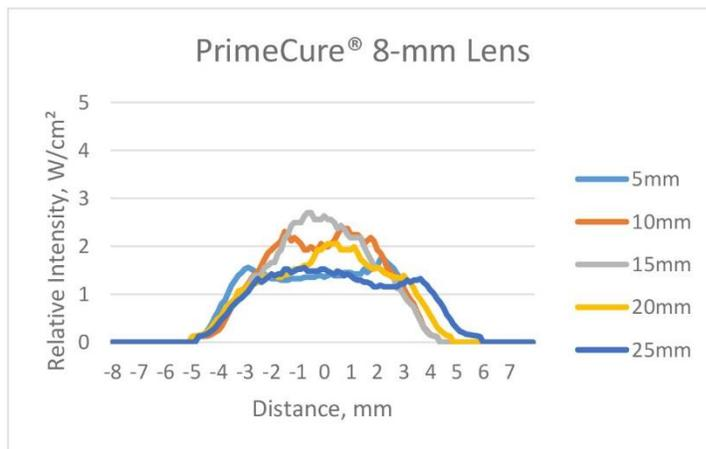
\*Curing Area Data taken using Fuji UV Light Distribution Mapping System and normalized to ACCU-CAL™ 50 LED Radiometer.
