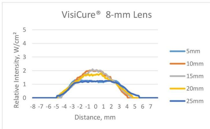
\*Curing Area Data taken using Fuji UV Light Distribution Mapping System and normalized to ACCU-CAL™ 50 LED Radiometer.
